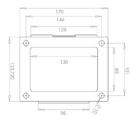
Wall plate's wall mount for Solarfox® SF-300 43" to 75"
